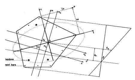
Fig. 5 Homogenized cross-section
