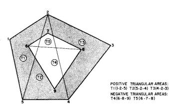
Fig. 2 Description of a section by triangles
