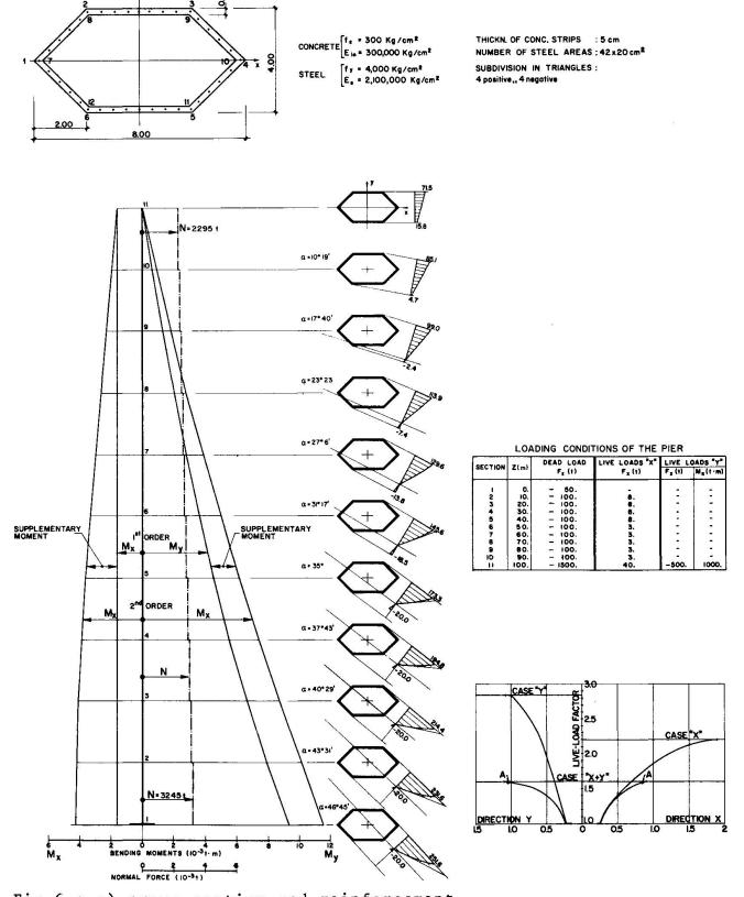
Fig.6: a) cross section and reinforcement
