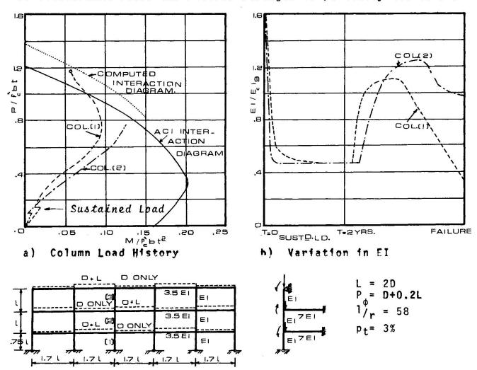
Fig. 5. Example of Behaviour of Columns in a Structure
