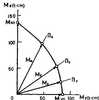
Fig. 4(c) Radial ultimate moments on final direction of eccentricity
