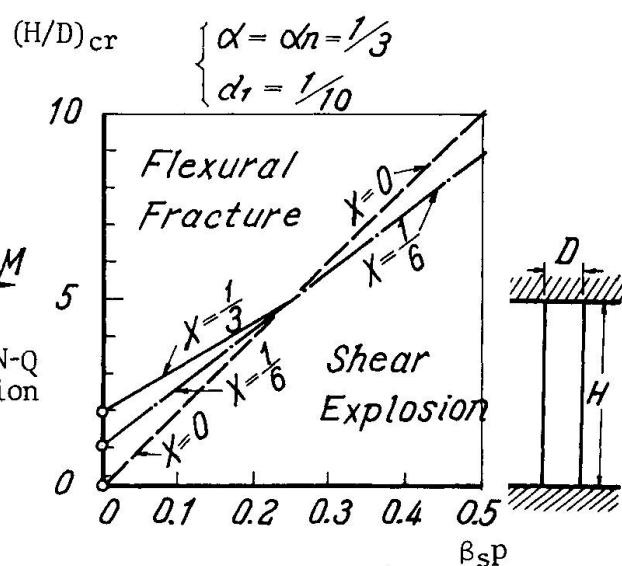
Fig.14 Critical Height to Depth Ratio
