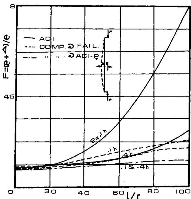
Fig. 3. Comparison of Moment Magnification
