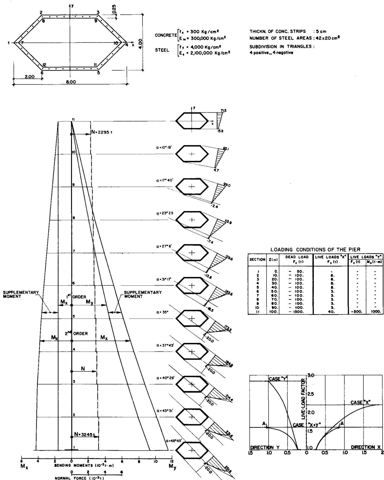
Fig. 6 : a) cross section and reinforcement
