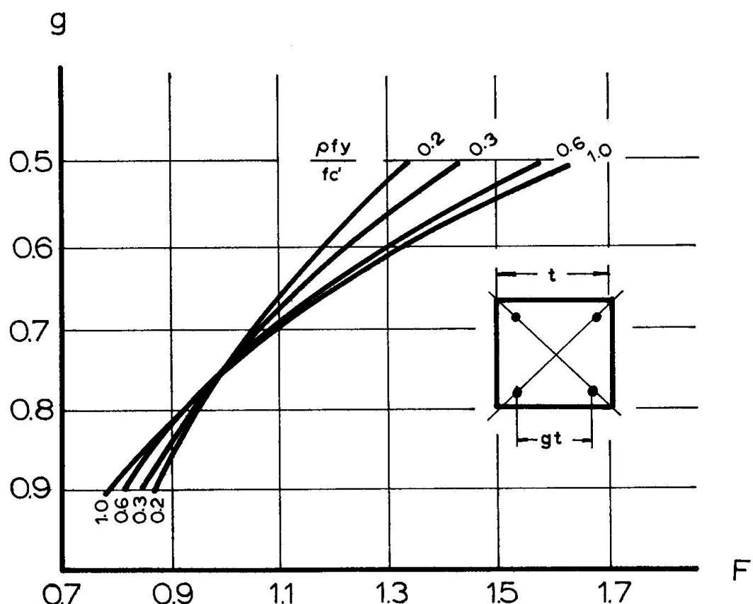
Figure 2 Factor  $F$  to modify results with a cover ratio  $g=0.75$  to any other cover ratio
