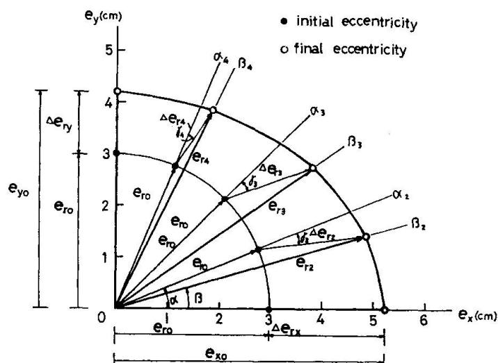
Fig. 4(a) Initial and final eccentricities projected on the  $e_x$ - $e_y$  plane
