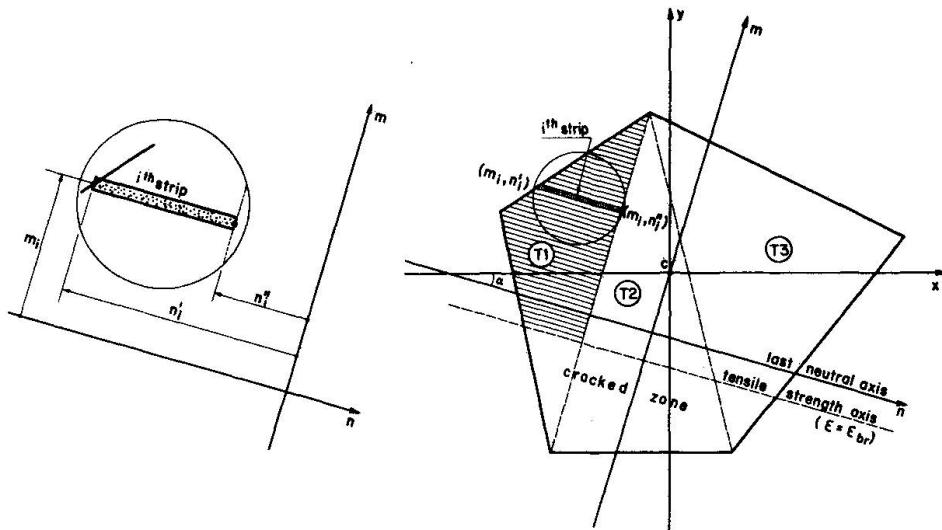
Fig. 4 Automatic discretization of the concrete area in each step
