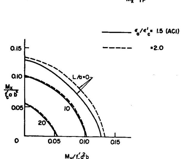
Fig. 11 Interaction Curves: Minimum Percentage of Steel
