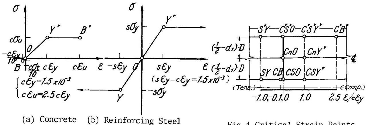
(a) Concrete (b) Reinforcing Steel
