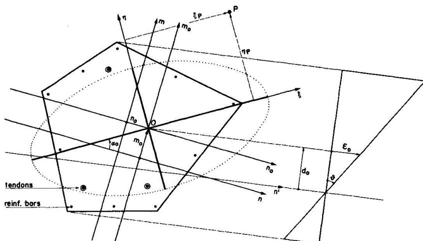
Fig. 5 Homogenized cross-section
