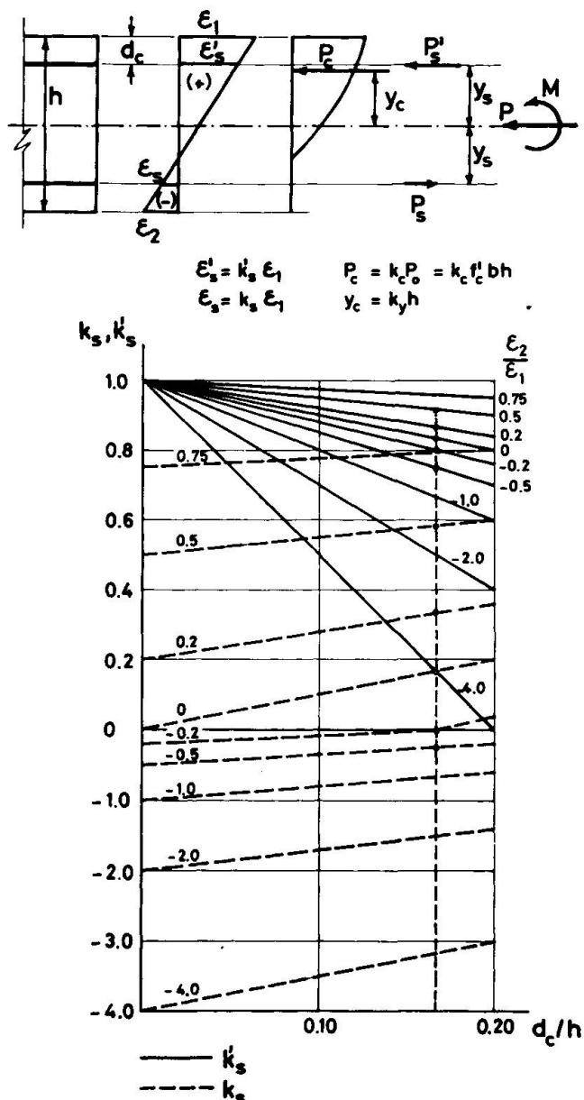
FIG. 4: COMPUTATION OF INTERNAL FORCES;
