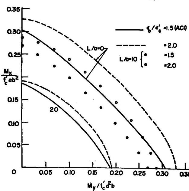
Fig. 10 Interaction Curves: Maximum Percentage of Steel
