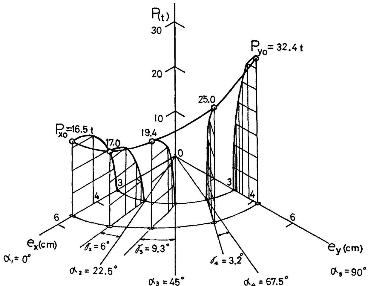
Fig. 3 Load-eccentricity relationships at the center section of biaxially loaded columns
