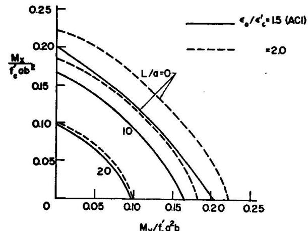
Fig. 9 Interaction Curves: Maximum Steel Quality Effect
