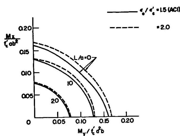
Fig. 8 Interaction Curves: Minimum Steel Quality Effect
