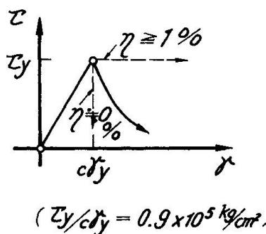
Fig. 7 Shear Stress - Strain Relationships of Concrete
