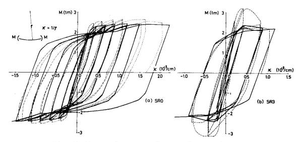
Fig. 5 Moment-Curvature Curves of SR Series
