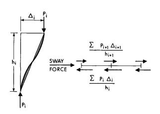
Fig. 8 Calculation of Sway Force
