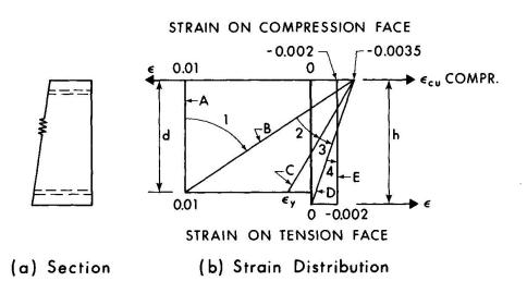
A - Pure Tension Failure
