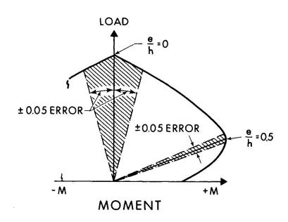
Fig. 5 Effect of Error in Eccentricity
