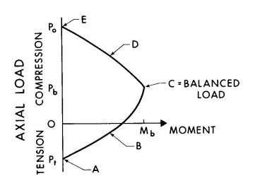
Fig. 2 Interaction Diagram
