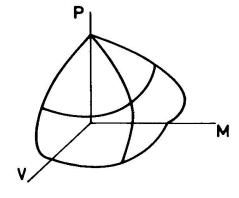
Fig. 6 M-P-V Interaction of a Column
