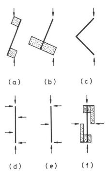
Fig. 3 Testing Methods of a Column
