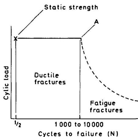
Fig. 2 FATIGUE RUPTURE CURVE FOR PULSATING TENSILE LOAD
