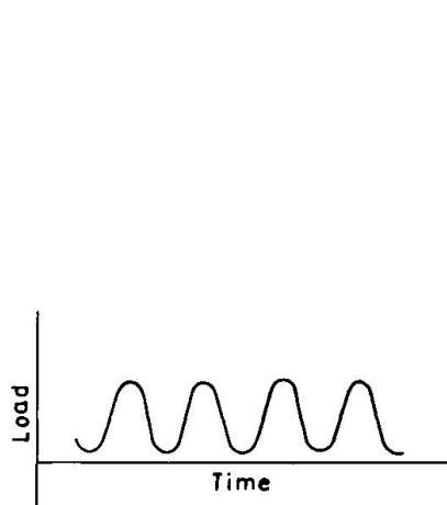
Fig. 1 PULSATING TENSILE LOAD
