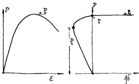
Fig.1 Stress-strain diagram and volume-strain-stress diagram
