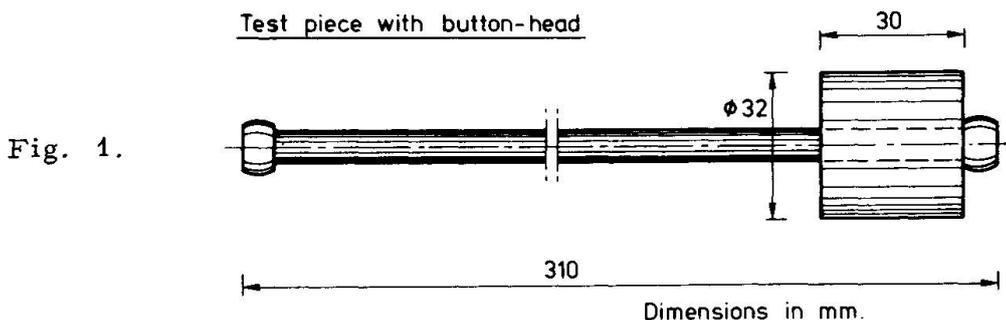
One prestressing system tested in our laboratory used button heads on the wires (see Fig. 1). These heads were made by pressing the ends
