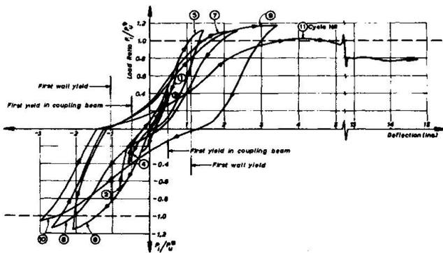
Fig. 3 Load - roof displacement relationship for walls with conventionally reinforced beams (above) and diagonally reinforced coupling beams (below) ( $P_i$  = applied load) ( $P_u$  = theoretical ultimate load)
