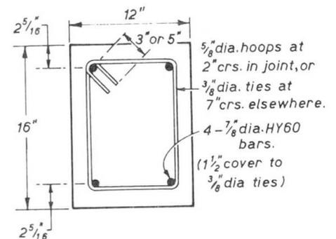
Fig. 4 Column Section of Units 1, 2 and 3 (1" = 25.4 mm).
