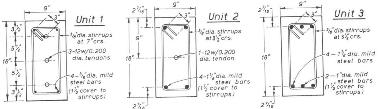
Fig. 5 Beam Sections (1" = 25.4 mm)
