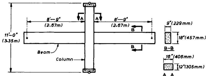
Fig. 1 Dimensions of Units 1, 2 and 3
