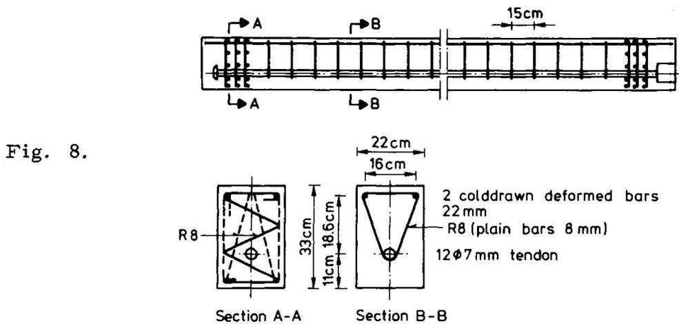
In three of the beams the cable duct was grouted whereas the duct was left ungrouted in the remaining three. The beams were subjected to a fatigue load in bending (see Fig. 9).
