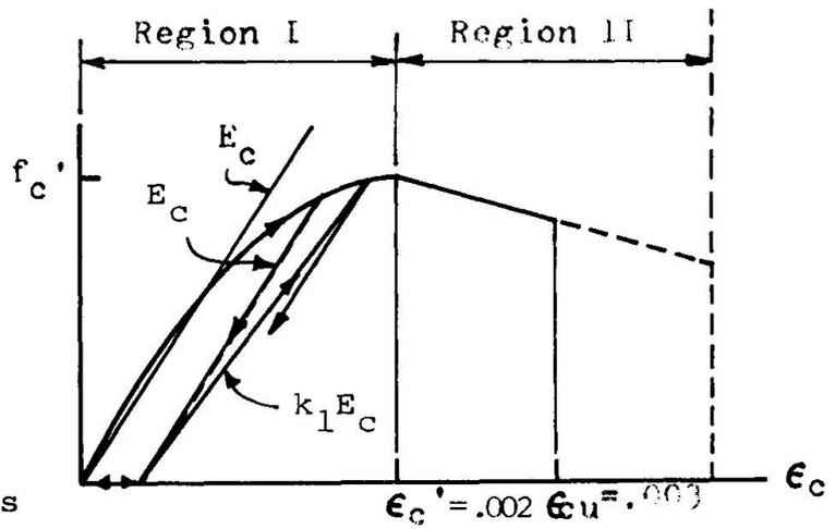
Figure 4 - Hysteresis Loops for Concrete
