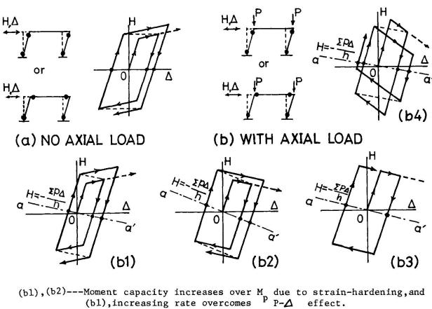
(b1), (b2)---Moment capacity increases over M due to strain-hardening, and (b1), increasing rate overcomes P P-Δ effect. (b2), P -Δ effect overcomes increasing rate.
