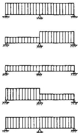
Fig.1 Loading scheme for the two span beams
