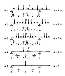
Fig. 3 Placing of the hydraulic jacks, cf tab. 1
