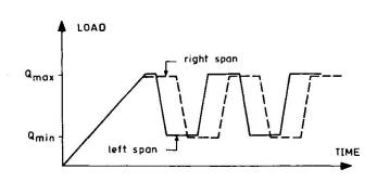
Fig.1 Loading scheme for the two span beams
