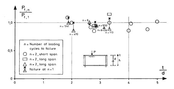
Ratios of failure load under repeated loading to failure load under Fig.2. monotonous loading.
