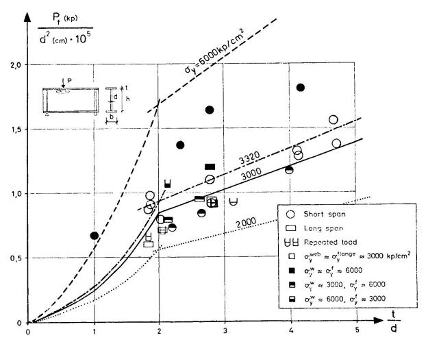
Fig. 3. Failure loads (crippling) for different steel qualities.
