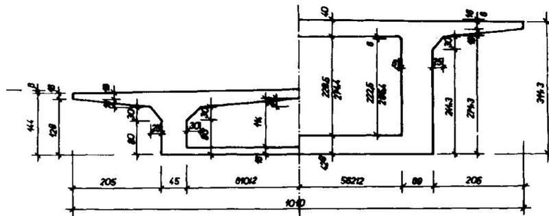
Fig.2 A scheme of cross-section of the bearing structure of the bridge Kollárovo.
