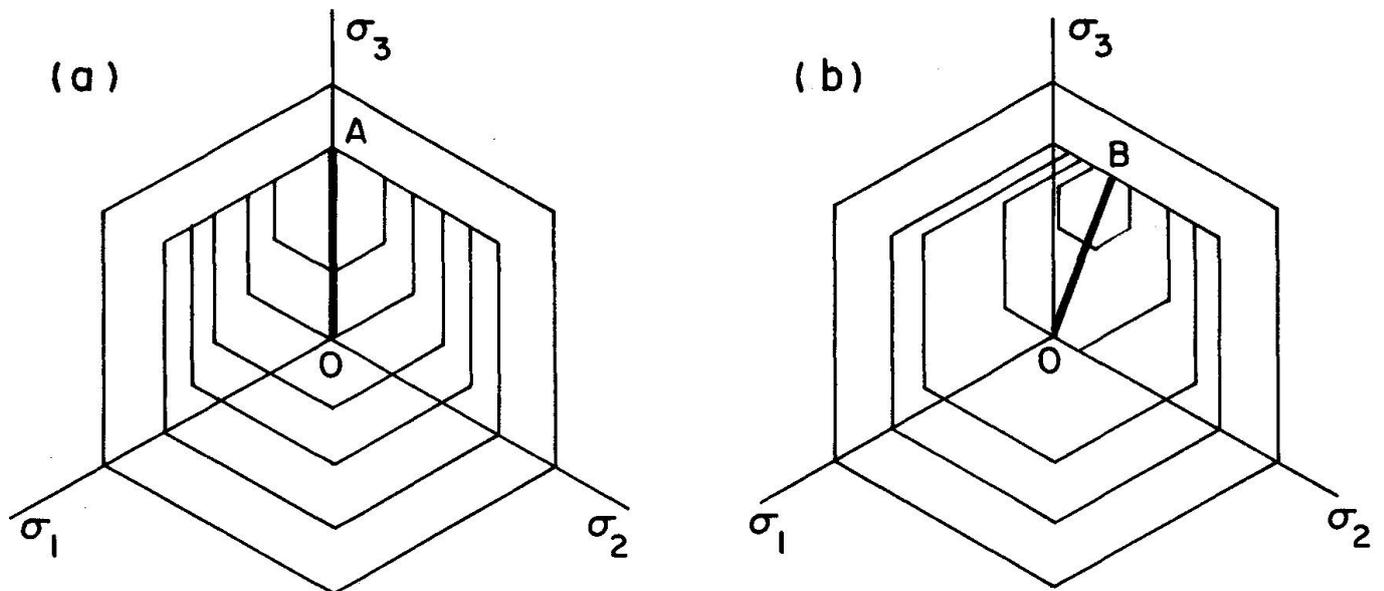
FIG. 2. Fields of hardening moduli after plastic loading
