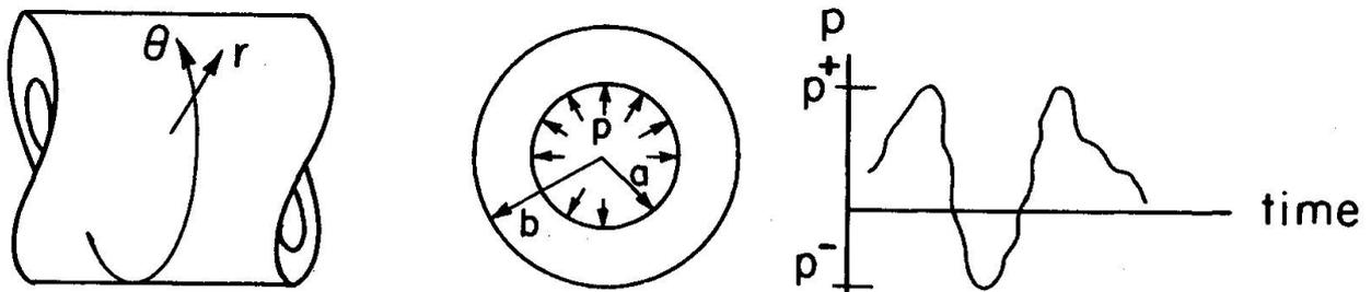
FIG. 3. Thick walled cylinder under cyclic pressure
