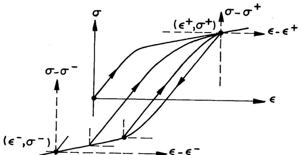
FIG. 1. Uniaxial stress-strain curve and steady-state hysteresis loops
