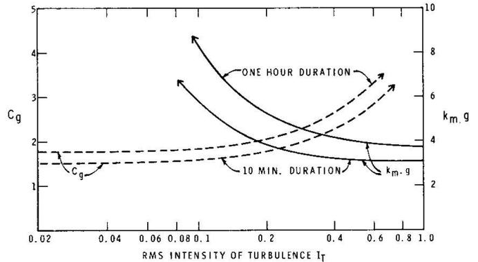
Figure 3: Gust Factors For Glass - Stationary Gaussian Loading
