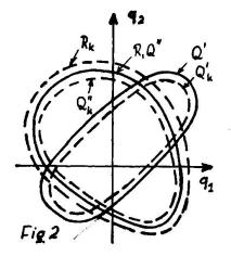
possible characteristic boundaries,  $Q'_k$  and  $Q''_k$ ). A first problem is the following: how to define a characteristic or a design boundary for loadings? The most natural answer could be: choosing it to be homothetical to the characteristic boundary  $R_k$ . But is this answer whenever possible the right one?
