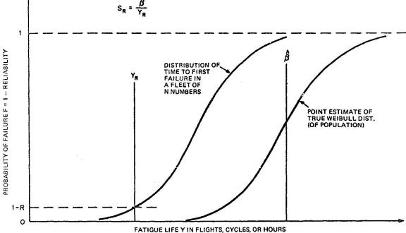
FIGURE 1 SCHEMATIC REPRESENTATION OF RELIABILITY PLAN
