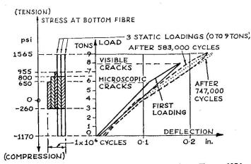
Fig. 4.—Load-deflection Diagram: Fatigue Tests, 1954.
