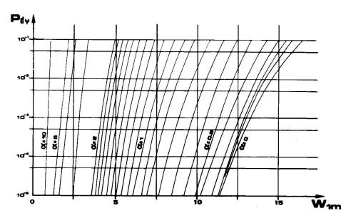
Fig. 4: Upper bound probability  $P_{d\psi}$  vs. load parameter  $W_{1m}$  ( $\alpha = W_{2m}/W_{1m}$ )
