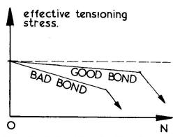
Fig. 7 Reduction in Tension stress during Fatigue.
