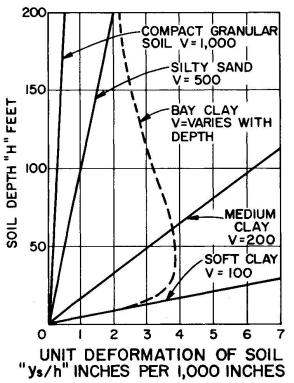
SHEARING DISTORTION OF GROUND BART DESIGN EARTHQUAKE
