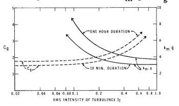
Figure 3: Gust Factors For Glass Stationary Gaussian Loading
