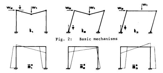
Fig. 3: Self-equilibrated diagrams of bending moment
