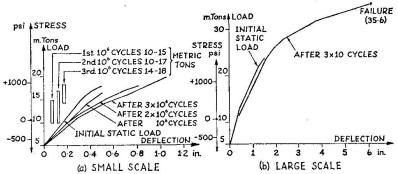
Fig. 3 ——Load-deflection Diagram: Fatigue Test, Composite Slab, Liège, 1951.
