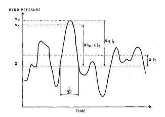
Figure 1: Wind Pressure Representation for Cladding Design
