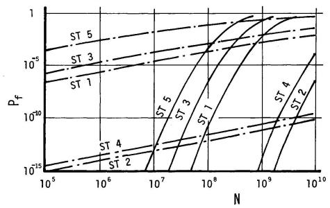
Fig. 4 Probability of Failure of Main Girders
