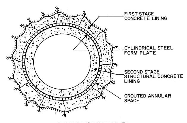
DEZ DAM PRESSURE TUNNEL SCHEMATIC CROSS SECTION
