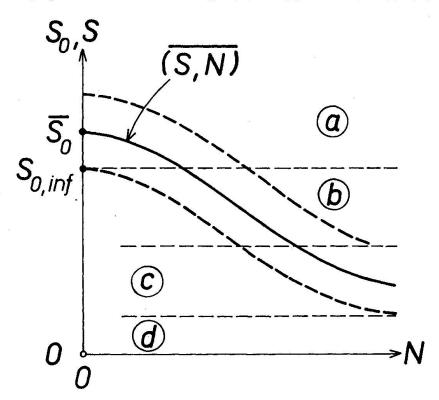
Fig.1. Fatigue ranges: (a) low-cyclic, (b) middle-cyclic, (c) high-cyclic,
