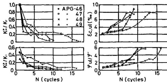
Fig. 7 Degradation of flexural stiffness  $K_w/K_i$ , and development of compressive extreme fiber strain  $\epsilon_{c,ul}$  of concrete and ductility factor  $\psi_{u,p}/\psi_p'$  at the peak load against the load number.
