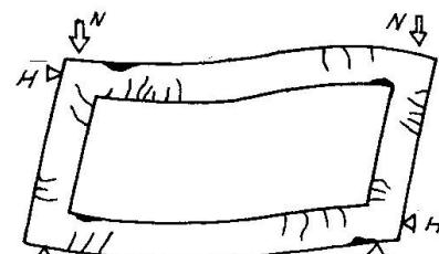
Fig. 3 (b)-4\* Cracking Patterns
