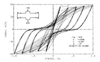
Fig. 6 Inelastic F -  $\Delta$ Hysteresis Loops
