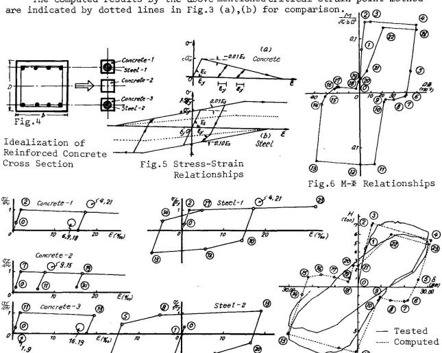
Fig.8 Process of Stress-Strain Relationships
