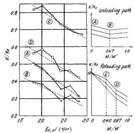
Fig. 3 Degrading flexunal stiffness K/Ko against the compressive extreme fiber strain Ec, ul of concrete at the beginning of unloading.
