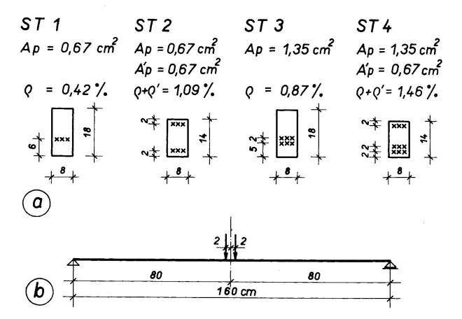
Fig.1. (a) Cross-section of specimens (b) Test scheme
