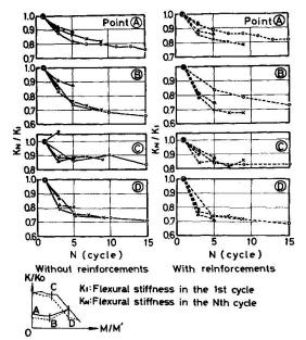
Fig. 5 Degrading flexural stiffness  $K_N/K_I$  against the load number.
