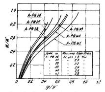
Fig. 1(8) Non-dimensional moment-curvature curves
