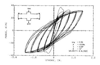
Fig. 5 Inelastic F -  $\Delta$ Hysteresis Loops (Beam 9)
