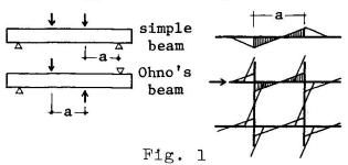
of the authors, at the RILEM Symposium of 1957 in Stockholm. By use of this loading method, the actual conditions of stress and deformation of members in frames subjected to lateral loads can be reproduced in the testing specimens as shown in Fig.1.
