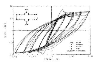
Fig. 4 Inelastic F -  $\Delta$ Hysteresis Loops (Beam 5)
