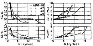
Fig. 7 Degradation of flexural stiffness Kn/Ki, and development of compressive extreme fiber strain Ec,ul of concrete and ductility factor Yul/9" at the peak load against the load number.
