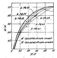
Fig. 1 (C) Non dimensional moment-curvature es during reloading stage after complete unload.
