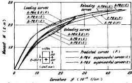
Rg. 4. Prediction of mament-curvature curves of prestnessed concret beams under repeated loadings.
