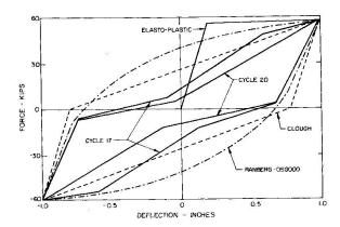
Fig. 13: Effect of Shear Pinching
