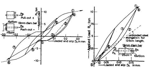
Fig. 8. COMPUTED BEHAVIOR OF THE PULL-OUT SPECIMEN [References]
