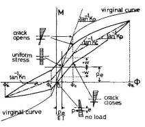
Fig. 10 Proposed model of N-th cycle moment-curvature curve of prestressed concrete beam under reversed flexural loading. (Φ<sub>k</sub> Φ<sub>k</sub> :specified constant curvature amplitudes )
