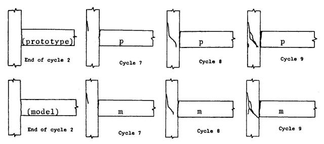
Fig. 3 - Crack patterns for Prototype I-A and model A3 at peak downward loadings (major cracks only)
