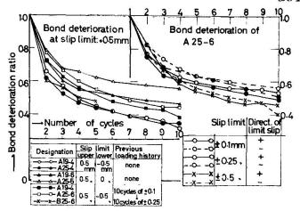
Fig. 5. THE BOND DETERIORATION RATIO (RS Tests)
