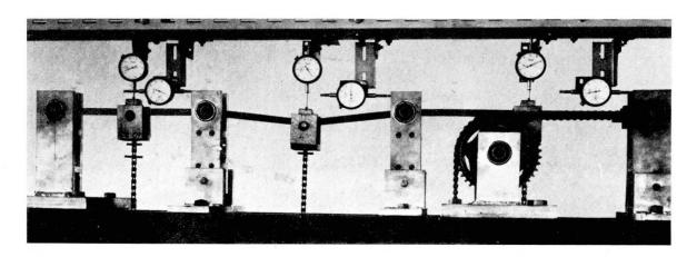
Fig 3. Apparatus for three-span tests
