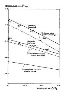
Fig 10. Three-Span Beam. Axial Load 669lb Fig 11. Three-Span Beams. Failure Loads
