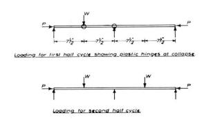
Fig 1. Loading cycle for two-span beams
