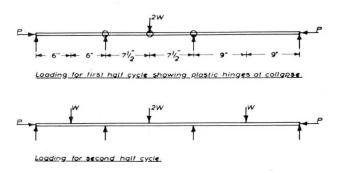
Fig 2. Loading cycle for three-span beams
