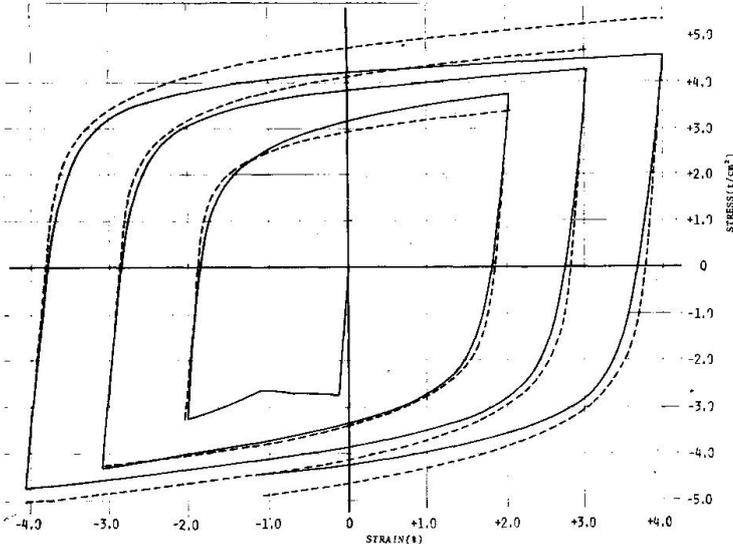
Fig. 5. COMPARISON OF EXPERIMENTAL AND APPROXIMATE STRESS-STRAIN CURVES
