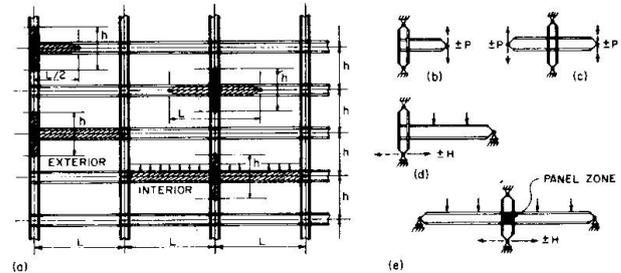
Fig. 1: Moment-Resistant Frame and Subassemblages
