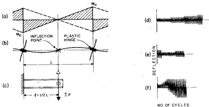
Fig. 3: Cantilever Idealization and Programs of Cycling
