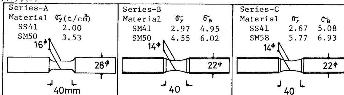
Fig.4. Test Specimens ( $\sigma_y$ =yielding stress,  $\sigma_B$ =breaking stress)
