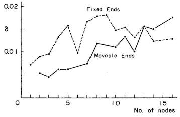
Fig. 7 Damping vs. Modes of Suspension Bridge Model
