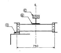
Fig. 8 Cross Section of Model Girder
