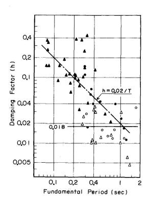
Relation between Damping and Fig. 3 Natural Period for Horizontal Fundamental Mode of Vibration (A: Foundations and ordinary piers, ◆: Bridges and ordinary piers, △: Tall piers with height greater than 25 m, o: Bridges on tall piers)
