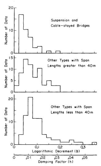
Fig. 1 Distribution of Damping Values of Bridge Superstructures
