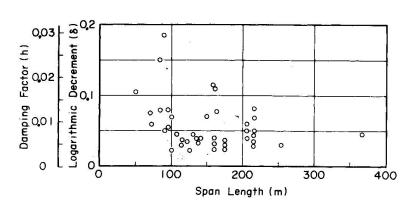
Fig. 2 Damping of Suspension and Cable-stayed Bridges vs. Span Length
