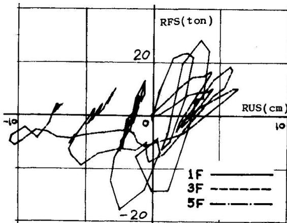
Fig.14 STORY SHEAR-STORY DISPLACEMENT DIAGRAM FOR VERNON(S82°E) EXCITATION
