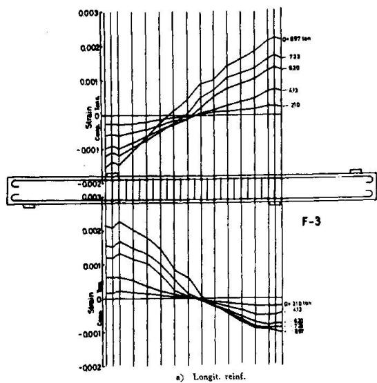
Fig. 16 Strain distributions of longitudinal steels and lateral ones
