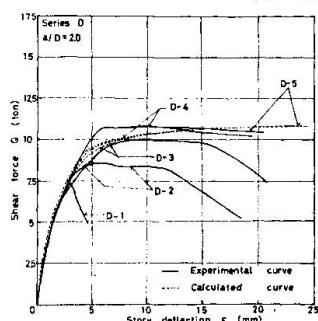
Fig. 7 Relationships between the shear force and the story deflection
