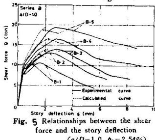
Fig. 5 Relationships between the shear force and the story deflection
