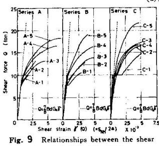
Fig. 9 Relationships between the shear force and the shear strain
