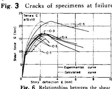
Fig. 6 Relationships between the shear force and the story deflection
