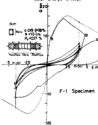
Fig. 11  $Q-\delta$ ,  $Q-\delta_{fi}$ ,  $Q-\delta_{sh}$  curves of F-1 specimen ( $a/D = 1.0$ )
