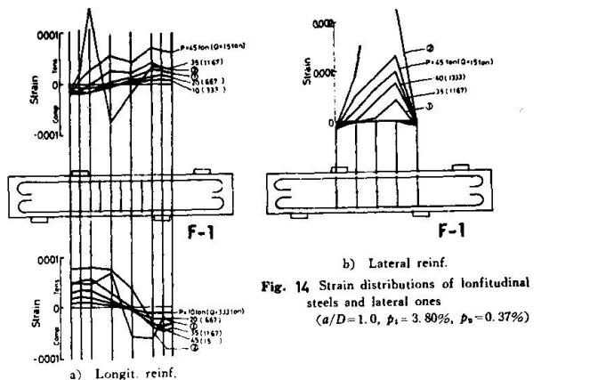
Fig. 14 Strain distributions of longitudinal steels and lateral ones
