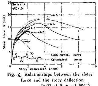
Fig. 4 Relationships between the shear force and the story deflection
