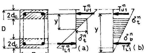
Fig. 19 Force equivalence of section
