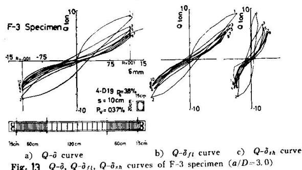
Fig. 13  $Q-\delta$ ,  $Q-\delta_{f1}$ ,  $Q-\delta_{sh}$  curves of F-3 specimen ( $a/D=3.0$ )
