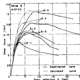
Fig. 8 Relationships between the shear force and the story deflection
