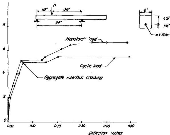
FIG. 3 - A TYPICAL LOAD-DEFLECTION CURVE FOR THE BEAMS
