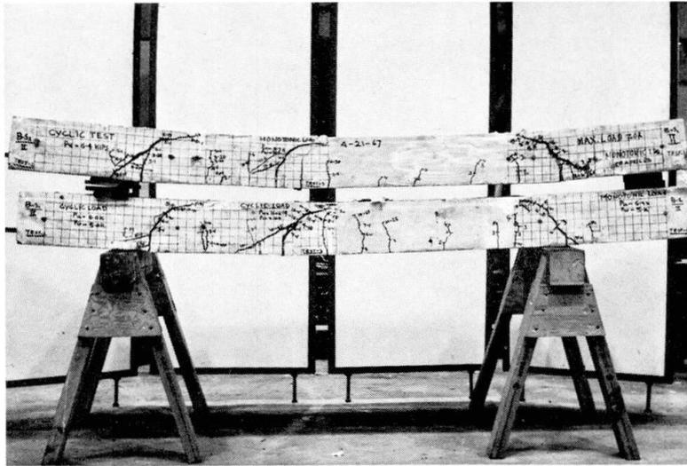
FIG. 4 — SHEAR FAILURE OF BEAMS
