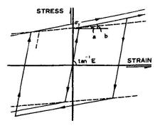
Fig. 3 Relation of stress-strain
