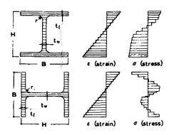
Fig. 4 Distribution of stress & strain
