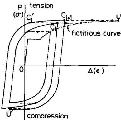
Fig.1 Stress-Strain Curve for Steel for Repeated Loading
