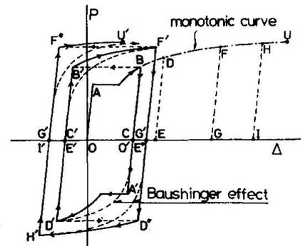
Fig.3 Construction of Cyclic Curve from Monotonic Curve
