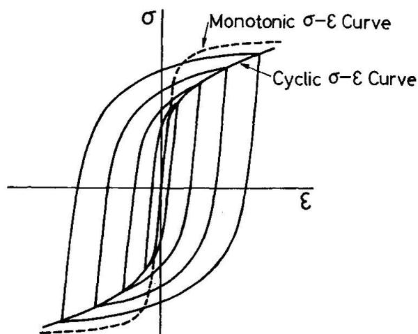
Fig. 7 Hysteretic Stress-Strain Relationship of Metal
