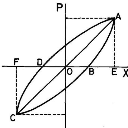
Fig. 3 Hysteretic Characteristics of a Nonlinear System
