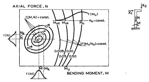
Fig. 3 - Bivariate densities of probability of loading and resistance.
