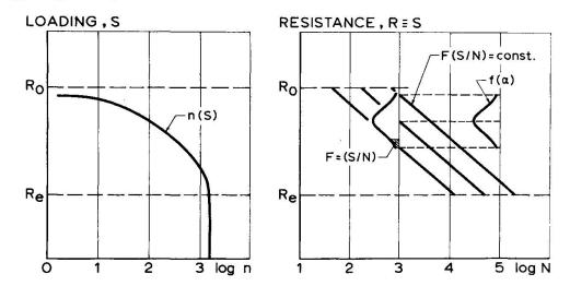
Fig. 14 - Diagrams indicating the number of loading cycles and fatigue life. latter case the probability of efficiency should be computed by a convolution of the distribution functions  $F_{\alpha}(\alpha(D))$  and  $F_{D}(D)$ .
