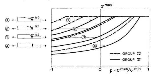
Fig. 15 - Design rules for fatigue, after (12).
