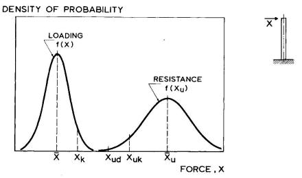
Fig. 1 - Densities of probability of loading and resistance.
