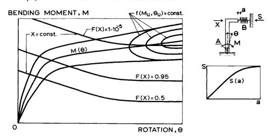
Fig. 6 - Non-linear statically indeterminate structure having random behaviour and acted on by a single random loading.
