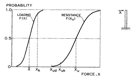
Fig. 2 - Distribution functions of loading and resistance.
