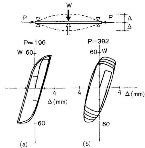
Fig. 9. Hysteresis Loops of Beam-Column under Repeated-Bending.
