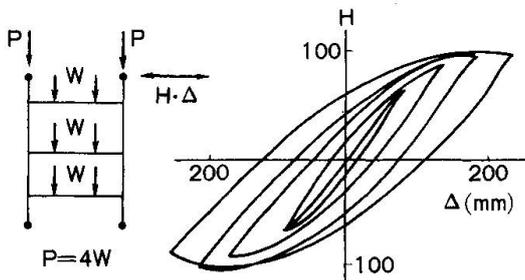
Fig. 17. Selected Load-Deflection Curves of a Frame under Repeated Horizontal Loading ( $P=4W$ ).
