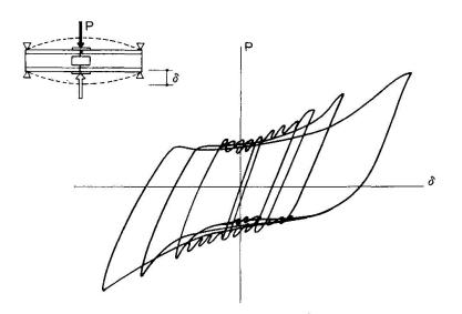
Fig. 11 P-δ curve of Wide-Flange Beam with High-Strength Bolted Joint.
