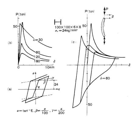
Fig. 7 Theoretical P-δ curves of a Bar under compression and Repeated Tension-Compression.
