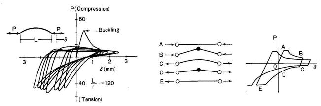
Fig. 5 Hysteresis Loops of a Bar under Repeated Tension-Compression.
