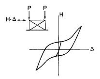
Fig. 25 S-Shaped Hysteresis Loop of a Braced Portal Frame under Horizontal Loading.
