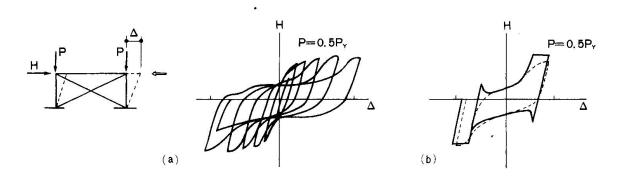
Fig. 24 Load-Deflection Curve of a Braced Full-Scale Portal Frame under Repeated Horizontal Loading
