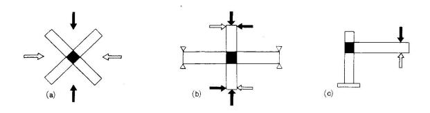
Fig. 12 Test Specimen of Beam-to-Column connection.
