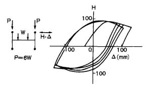
Fig. 18 Selected Load-Deflection Curve of a Frame under Repeated Horizontal Loading. (P=6W).
