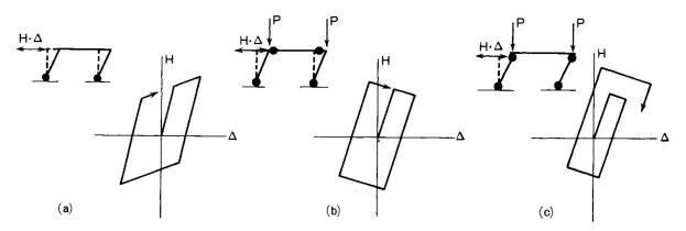
Fig. 21 Positive and Negative Bilinear Histeresis Curves of Portal Frames under Repeated Horizontal Loading.
