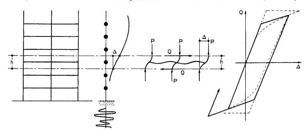
Fig. 14 Elastic-Plastic and Bilinear Type Restoring-Force Characteristics Used in the Seismic design.
