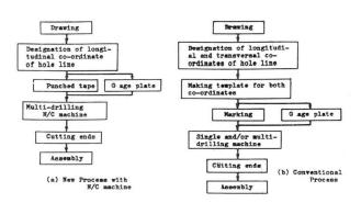
Fig. 4-2; Change in Preparation Process for H-shape brought by the Use of N/C Machine
