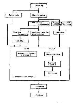
Fig. 5-2; Production System in High-rise Building Frame
