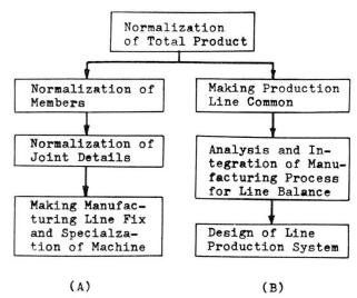
Fig. 2-3; Process to Mass Production System
