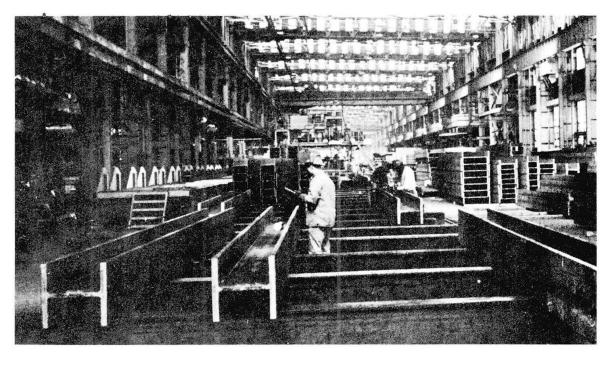
Fig. 11 Inspection Skids (Courtesy Inland Steel Company)
