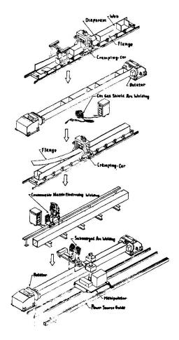
Fig. 3-2; Assembling Line of Box Colomn
