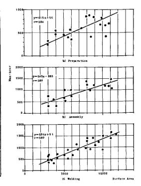
Table 3-1; Example of Analysis into Unit Work (Assembly of Tubular Structure)
