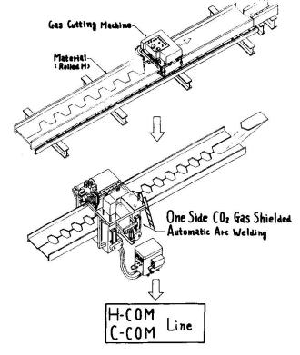
Fig. 5-1; Assemblying Line for Honeycomb Beam
