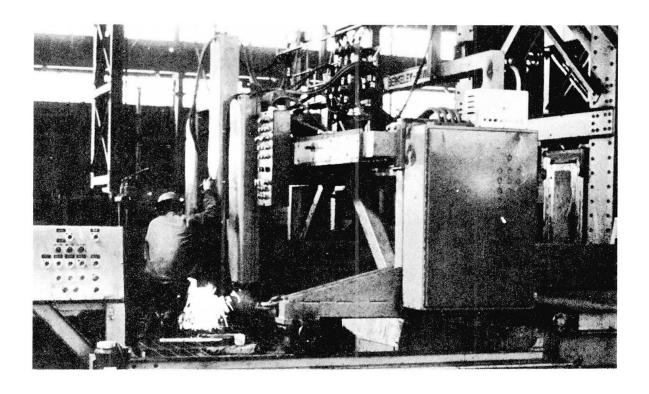
Fig. 10 Flame-Cutting to Length (Courtesy Inland Steel Company)
