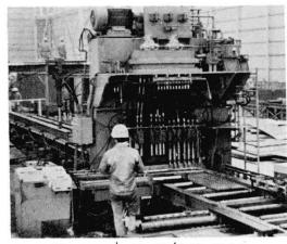
Photo. 4-5; N/C Drilling Machine for Splice Plate (S-COM)
