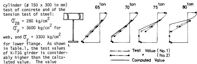
Fig.9 Stress Distribution in Inelastic Range
