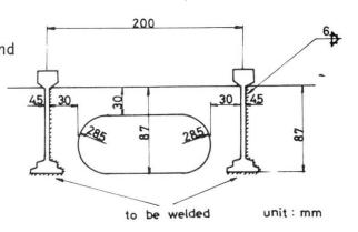
Fig.3 Punching Holes and Welding
