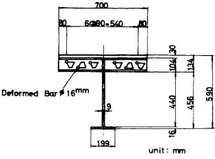
Fig.5 Cross Section
