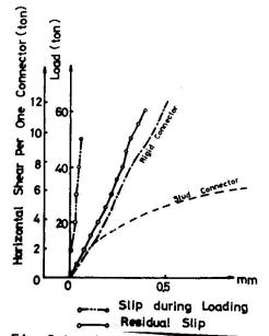
Fig.6 Load-Slip Curve
