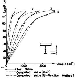
Fig.7 Load-Strain Curve at Span Center
