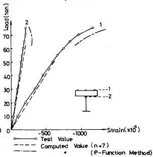
Fig.8 Load-Strain Curve at Span Center
