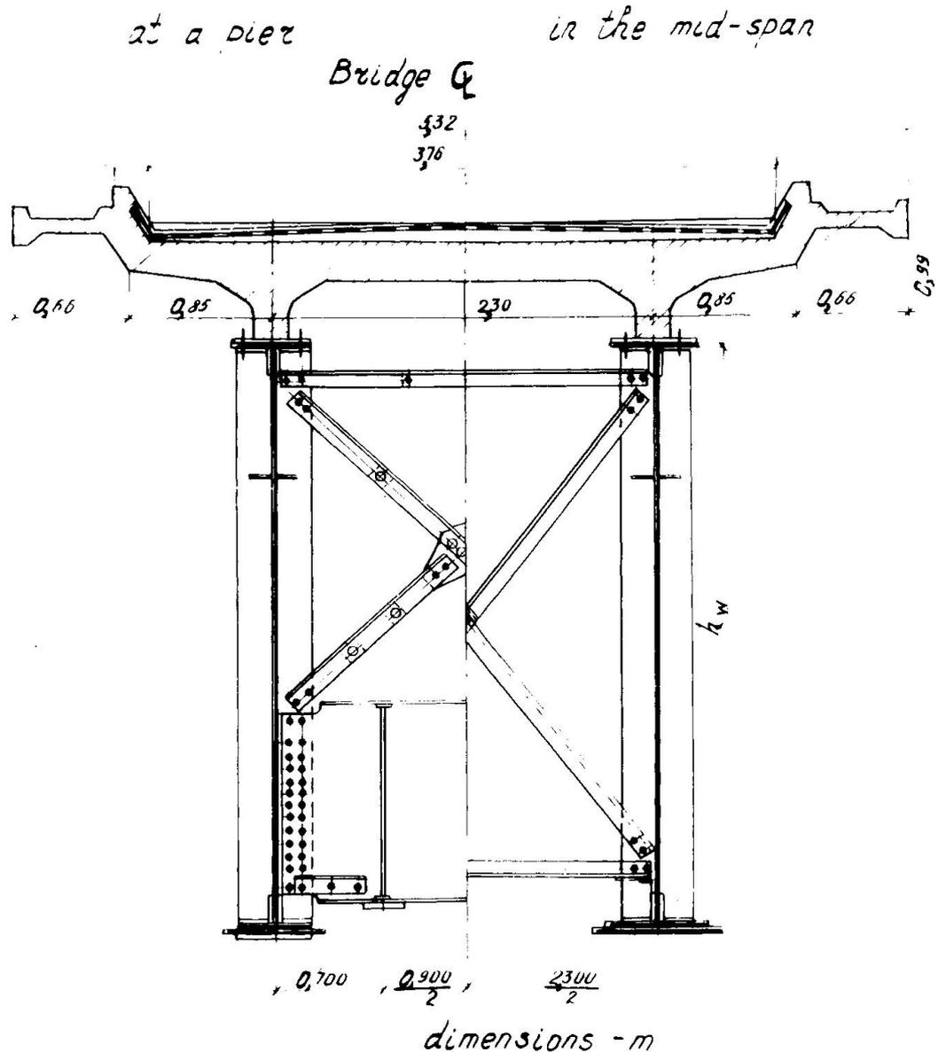
deck slabs. These are connected to the steel girders either using rigid studs, or high-strength bolts and epoxy-resin based glue; the latter being recognised in the USSR as the most efficient technique as much in terms of providing the connection reliability of the structure in service conditions as in terms of the convenience of including the precast deck slab into composite action with the steel girders during the cold seasons.
