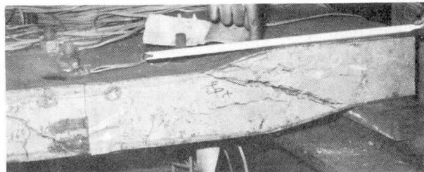
Photo. 6 Shear failure at a support
