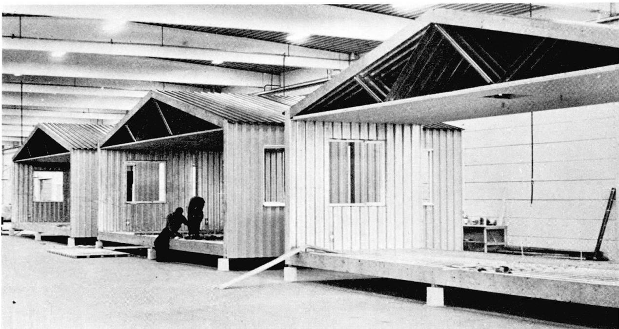
All sheet steel is galvanized to 30  $\mu\text{m}$  zink thickness and all outer surfaces are plastic coated with 200  $\mu\text{m}$  Organosol. The plate thickness is 0,9 mm and the height of the trapezium-profile pattern is 45 mm.
