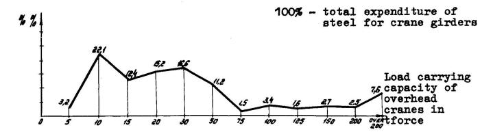
Fig. 4. Use of crane girders in per cent in terms of load carrying capacity of everhead cranes
