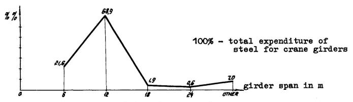
Fig. 3. Use of crane girders in per cent in terms of girder span
