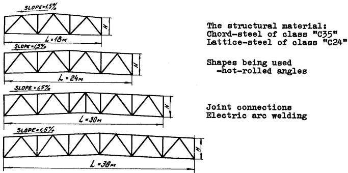
Fig. 5 Diagrams of standard roof trusses
