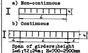
The structural material 1. Light and mean duty Chords-steel of class "C35". Wall-steel of class "C24"
