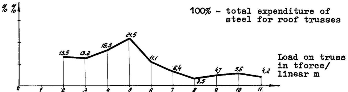
Fig. 2. Use of roof trusses in per cent in terms of load effected on the truss
