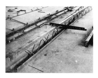
$Fig \ 14 \\$  Assembly of a complete column
