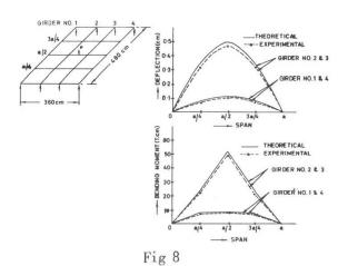
Deflection and bending moment curves for the interconnected beam
