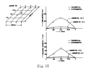
Deflection and bending moment curves for the interconnected beam with cast-in-situ slab
