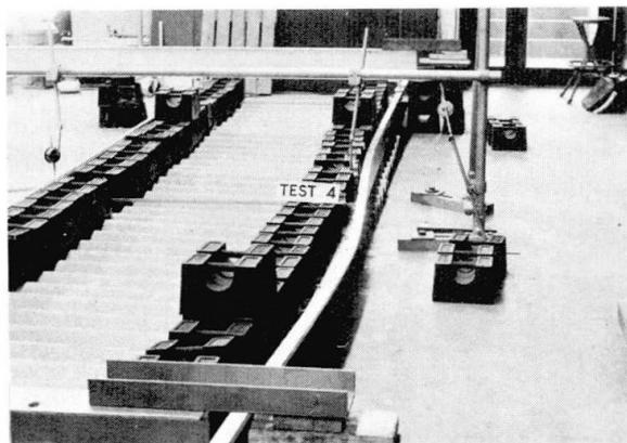
Fig 14      Reverse Loading Test on Purlin
