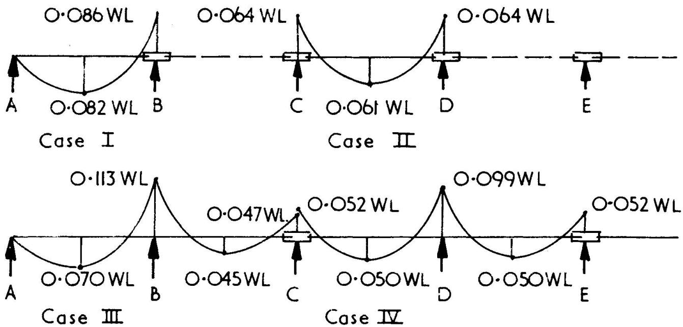
Fig 11 Bending Moment Diagrams for Purlins
