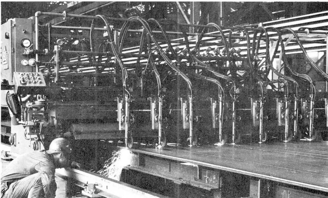
Fig. 6 Automatic Flame-Cutting (Courtesy Inland Steel Company)
