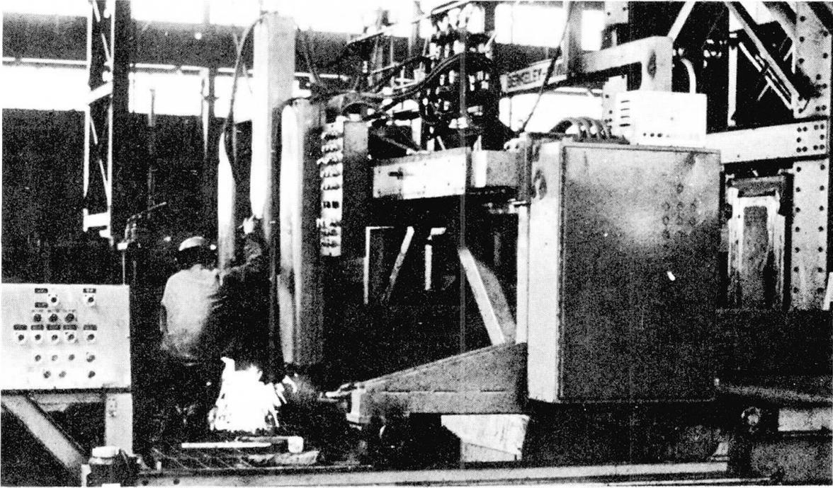
Fig. 10 Flame-Cutting to Length (Courtesy Inland Steel Company)
