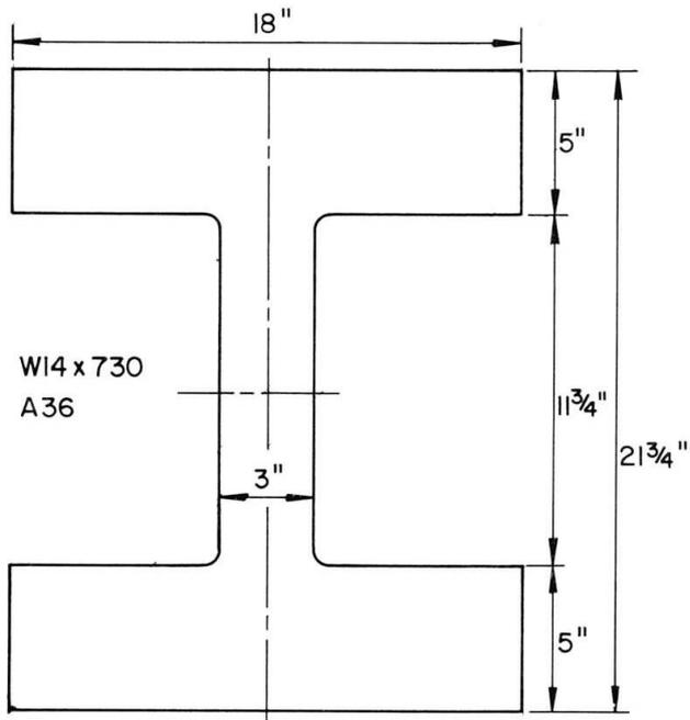
Fig. 3 Dimensions of Heavy Rolled Shape W14x730
