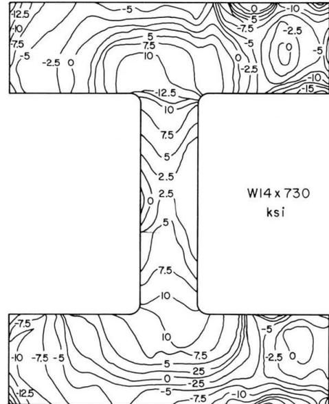
Fig. 4 Residual Stress Distribution in W14x730 Shape
