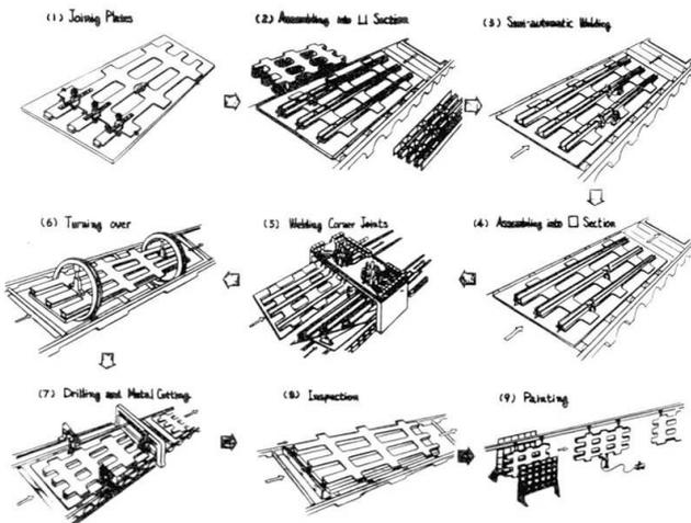
Fig. 2-2; Specialized Assembling Line for N.Y., WTC Building Column
