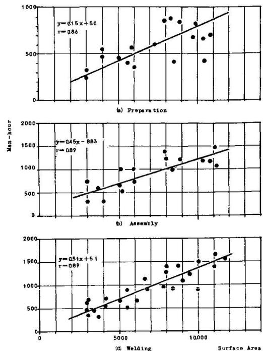
Fig. 3-3; Relation Curves of Man-hour/Surface Area (Truss)
