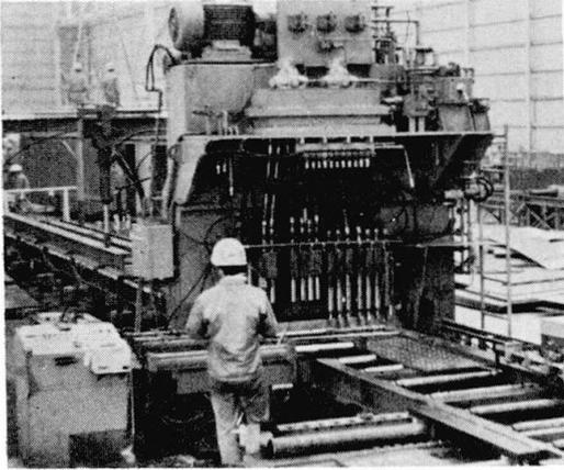
Photo. 4-5; N/C Drilling Machine for Splice Plate (S-COM)
