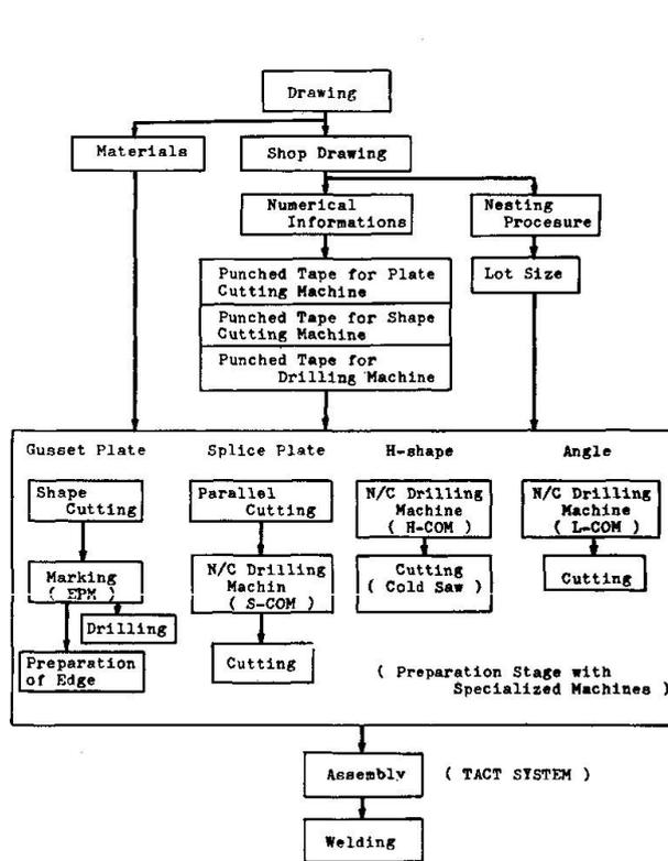
Fig. 5-2; Production System in High-rise Building Frame
