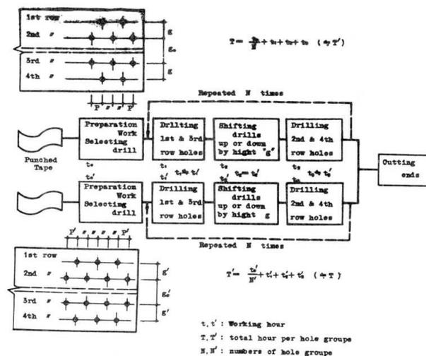
Fig. 4-3; Drilling Time per Hole Group When Drilled by N/C Machine
