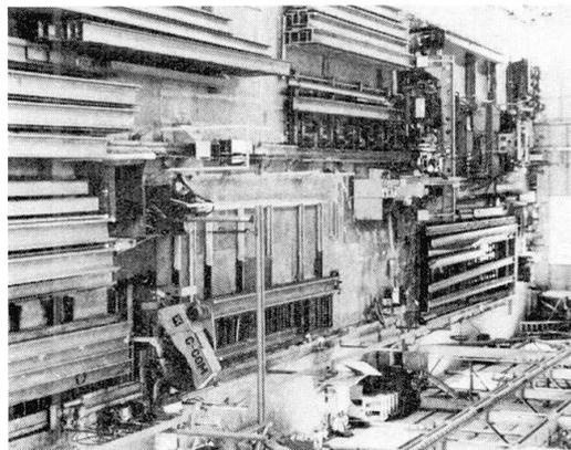
Photo 4-4; Drilling and Cutting Line for H-shape
