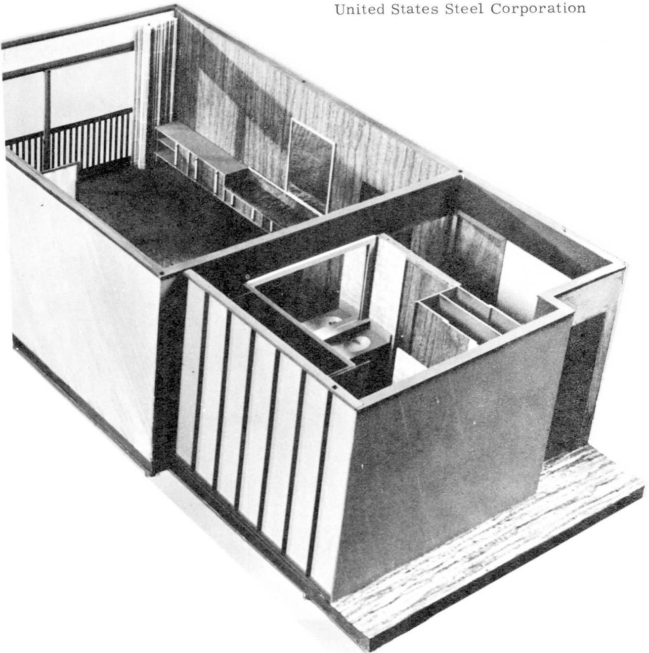
Republic Steel Corporation, a long time producer of building products, will soon enter the field of residential building systems with a single family detached residence. The principal material used in the residence construction will be steel. The residence has been designed for high volume industrial production yet it is flexible in appearance and arrangement.
