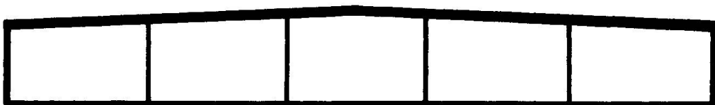
Beam and Column Width: 48' through 400' Height: 12' through 30'
