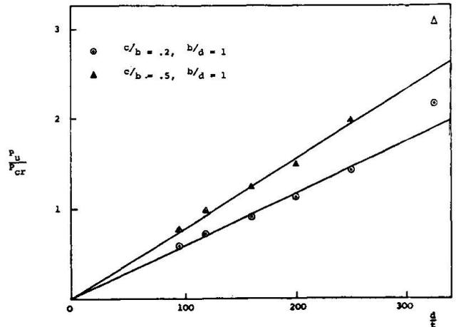
Fig. 11. Variation of the load ratio  $P_u/P_{cr}$  with the slenderness ratio ( $d/t$ ).
