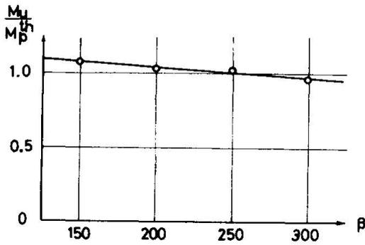
Fig. 5.  $M_u / M_p^{th}$  versus  $\beta = h/t_w$
