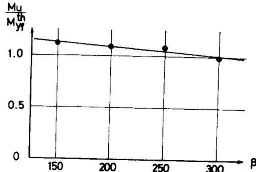
Fig. 6.  $M_u / M_{yf}^{th}$  versus  $\beta = h/t_w$
