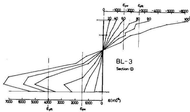
Fig. 4. Strain Distribution in Test Panel of BL-3 Girder
