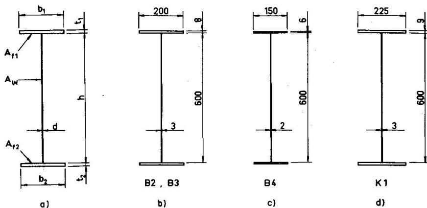
Fig. 2 a) Notations for cross section
