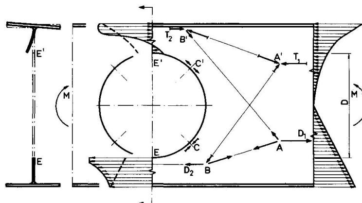
Fig. 12 Stress model for a girder with a circular web hole. Bending moment. torsional buckling, upward or downward vertical buckling and lateral buckling of the compression flange over the hole. Such restrictions are given in fig. 13.
