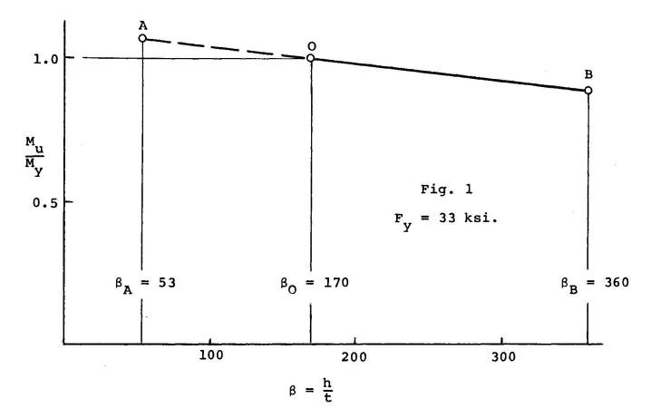
The essential features of Basler and Thurlimann's development of an equation for the ultimate bending moment, which accounts for stress redistribution, can be described with the assistance of Fig. 1, where the ordinate is the ratio of the ultimate moment to the moment required to initiate flange yielding,  $M_{tl}/M_{v}$ , and the abscissa is the web slenderness ratio,  $\beta$  = h/t.  $\beta_{\Delta}$  is the highest slenderness ratio for which the full plastic moment M  $_{
