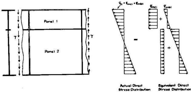
The critical stresses  $\sigma_{mc}$ ,  $\sigma_{mb}$  and  $\tau_m$  at which will cause buckling under their combined action occurs can be predicted with reasonable accuracy by equation (23).
